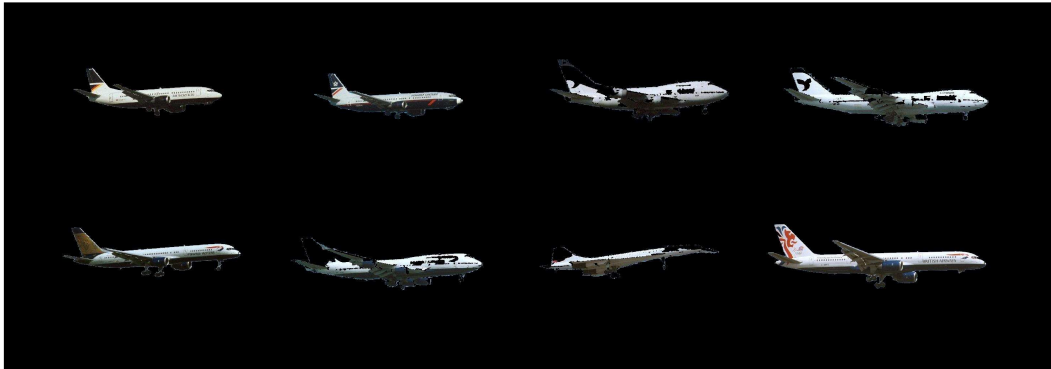
Figure 7.6: A set of regions obtained by a weakly-supervised approach ( a = Elongation ). This cluster is labeled with the visual concept StrongElongation . The good quality of the automatic segmentation is explained by the fact that the background of the associated non-segmented images is a clear sky.
